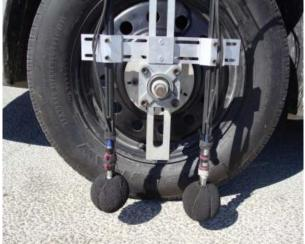
Figure 5-7: On Board Sound Intensity Measurement
