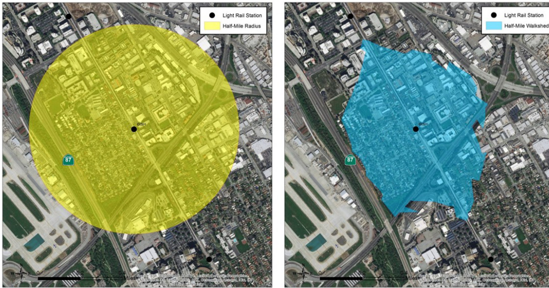
Figure 2-26. Comparison of Half-Mile Walkshed Area and Half-Mile Radius Around Gish Light Rail Station
